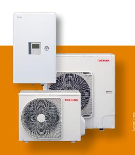
Air to water heat pumps in split design for leaving water temperatures up to +65°C, in the capacity range from 4 to 14 kW, for the preparation of hot or cold water. Combination of outdoor unit and hydrobox to supply all applications such as hot water tanks, fan coils, radiators or underfloor heating.
